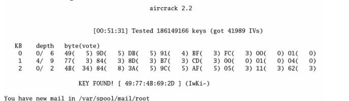
Figure 7: 64-bit key Capturing and Cracking.
