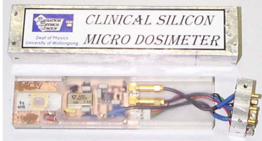
Figure 4.12. Probe assembly #2: PCB mounted electronics showing Fujitsu prototype microdosimeter, preamplifier and buffer amplifier. The board inserts into an aluminium box with the remaining air gaps filled by Lucite blocks.
