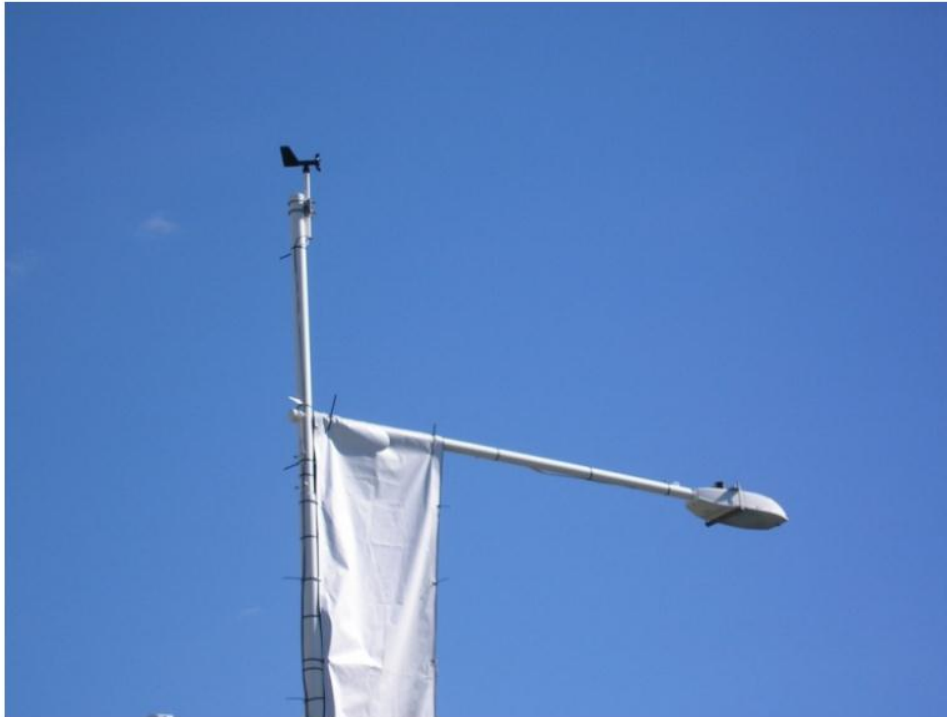
Figure 1. The Mt Oustley, Fairy meadow Standard Series Public Lighting Round Pole with vibration sensor and wind condition data logger installed.
