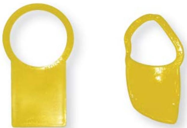
Figure 10 Normal and heat effected test tags
