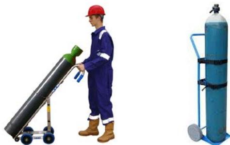
Figure 11 Mechanical handling devices
