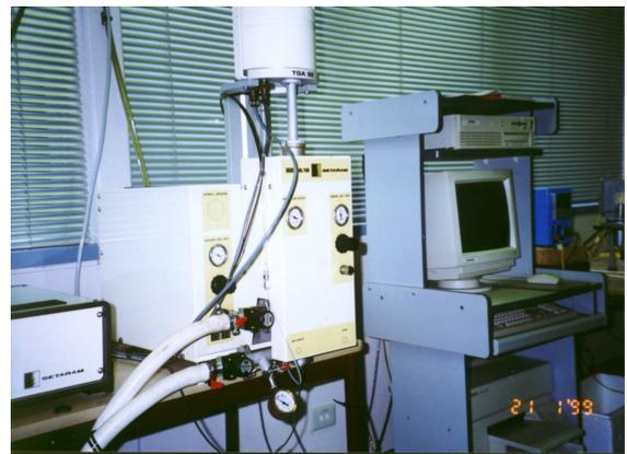
Simultaneous DTA/TGA to 1700°C
