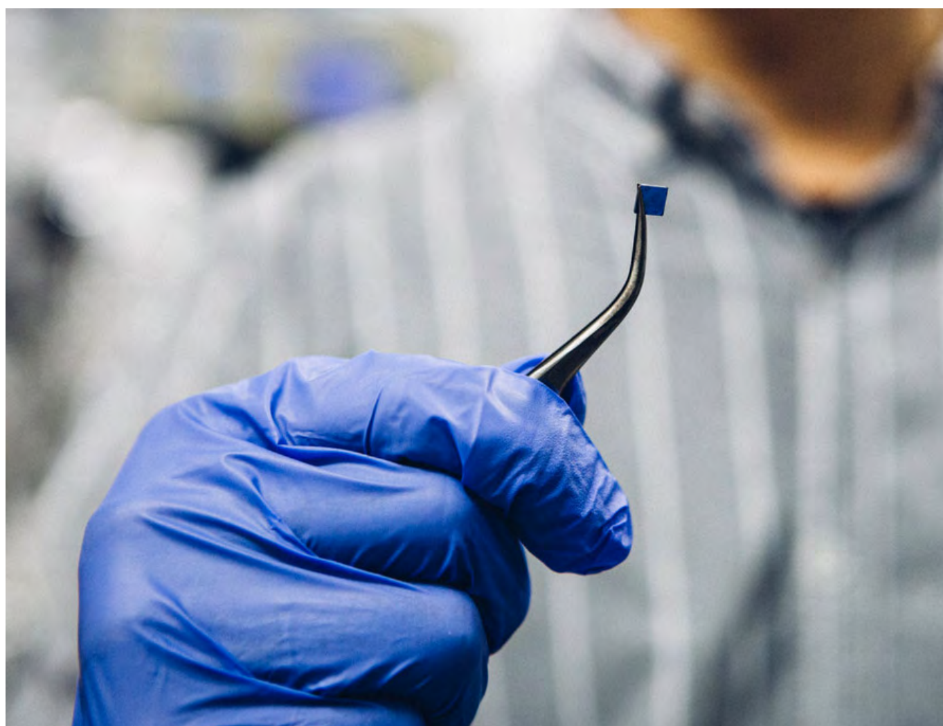
A high-performance titanium-oxide electrocatalyst for water splitting fabricated in collaboration with Beihang University.
