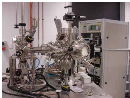
8T variable temperature scanning tunnelling microscope.
