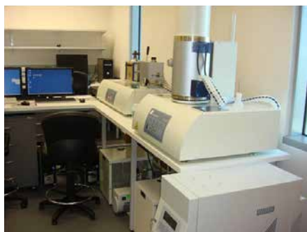
High temperature Seebeck coefficient, electrical conductivity, and thermal conductivity systems.
