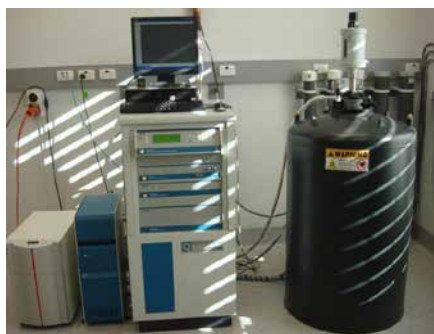
14T Physical Property Measurement System.
