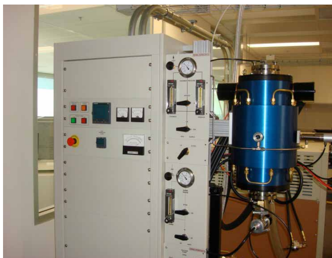
High vacuum, high temperature furnace (up to 3000°C).
