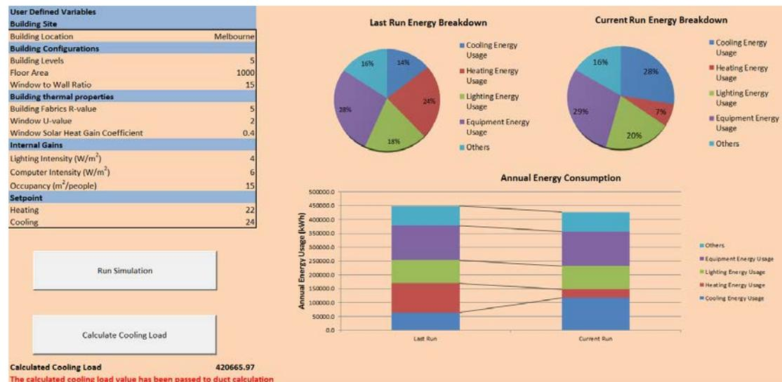
**Figure 4.1 - User interface of the building energy consumption estimation.**
