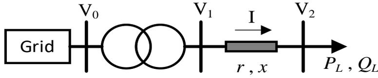
Fig. 4-3 Voltage drop in a distribution system
