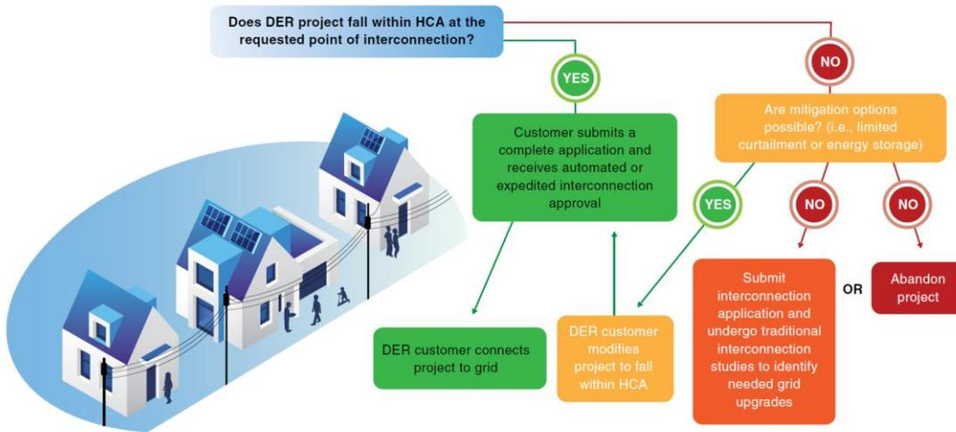
Fig. 5-4 DER connection use case for HC analysis [21]
