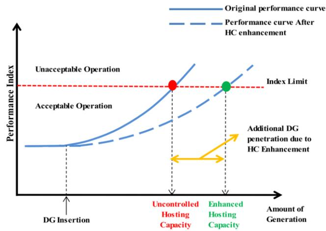
Fig. 5-2 HC concept and HC enhancement impact [20]
