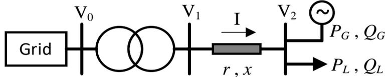
Fig. 4-4 Distribution system with load and renewable generation
