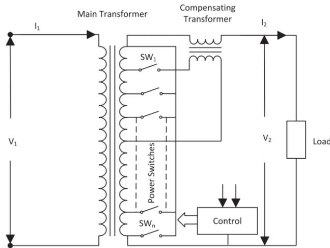
Fig. 6-2 Schematic of a fast on-load tap changer [8]
