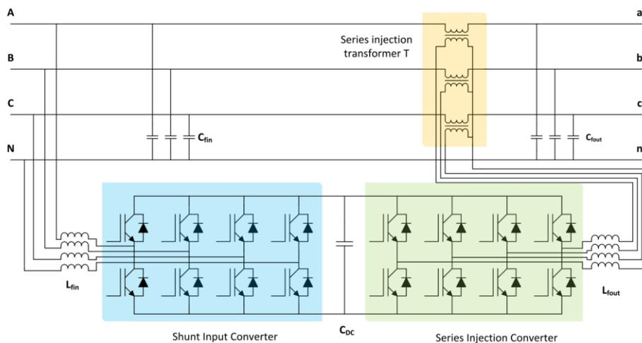
Fig. 6-5 Schematic of a UPFC connected to a DN [71]
