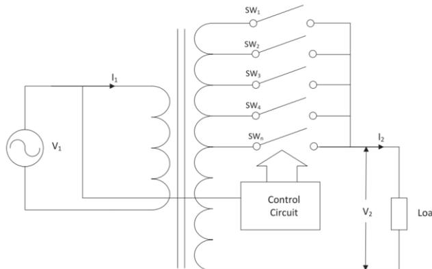
Fig. 6-1 Schematic of a typical on-load tap changer [8]
