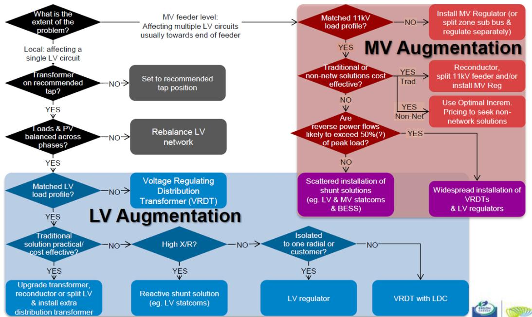
Fig. 6-7 Network options for mitigating voltage problems [86]
