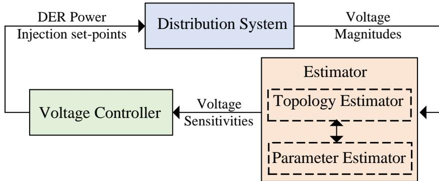
Fig. 8-2 A sample data-driven voltage regulation framework [101]
