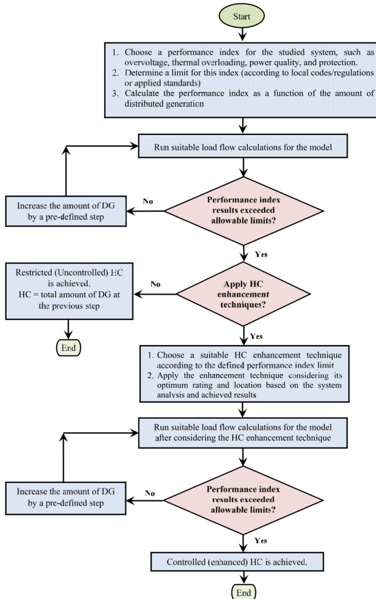
Fig. 5-3 HC assessment and enhancement procedure [20]
