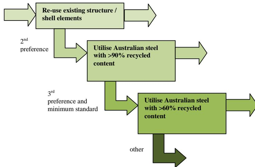
Steel should meet or exceed its required strength grade, and be permanently marked with this grade. A minimum of 60% of the steel used should be sourced from a contractor accredited by the Environmental Sustainability Charter of the Australian Steel Institute.
