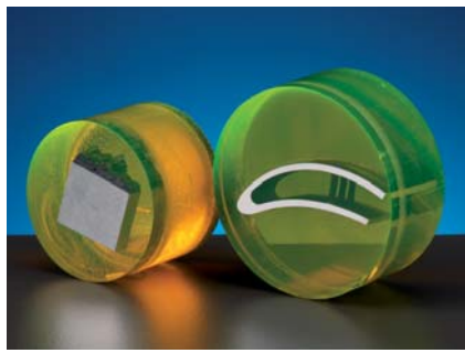
Steel components mounted with EpoFix and EpoDye
