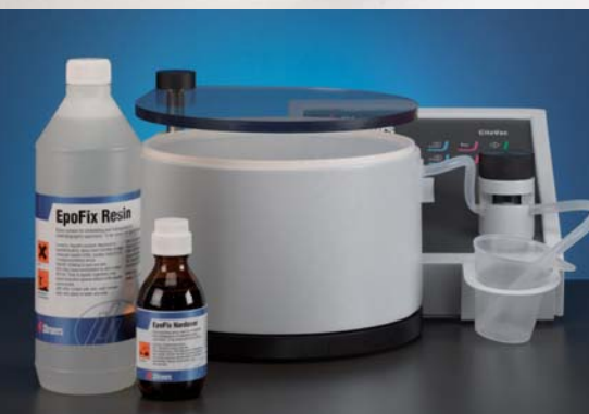
CitoVac with Struers impregnation material (EpoFix).
