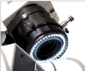
Viewing with full ring illumination
