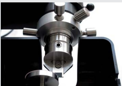
Sample holder attached on the alignment accessory. The micro-targets can be aligned during the process while observing with the stereo microscope.
